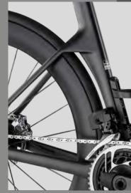
We knew pushing the envelope of the updated UCI limits on frame shapes could be tricky, but it was a challenge we ran to, rather than from. Again, borrowing lessons we learned from the Speedmachine, we expanded the horizontal profile in key locations like the head tube, bottom bracket, and seatstay junction. The resulting shapes not only look fast but enable the Teammachine R to respond more effectively across a wider range of yaw angles.
