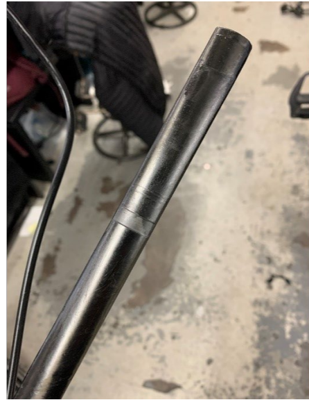
Marks on a flat steerer tube.
