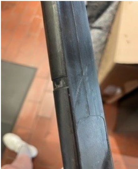
Deep wear on a flat steerer tube. This fork must no longer be ridden!
