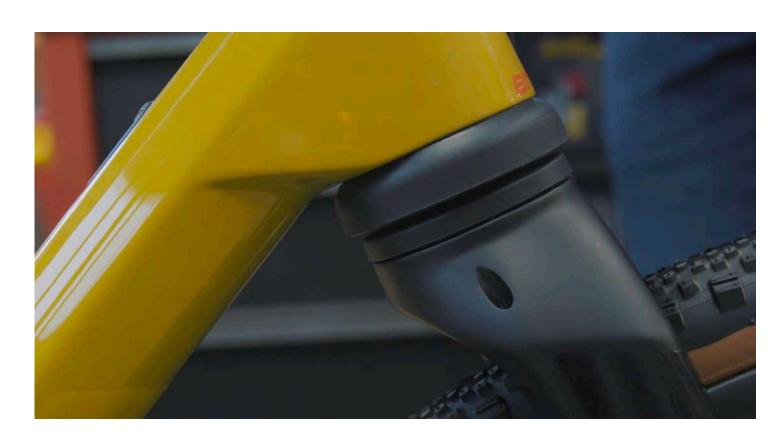
Make sure the suspension is full extended before tightening the top cap
