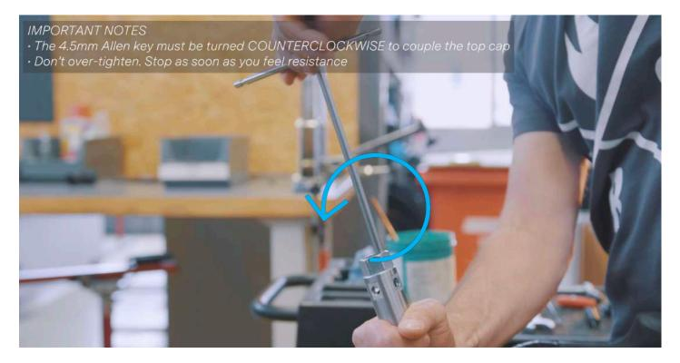
Couple the top cap with the piston shaft using the 4.5mm
