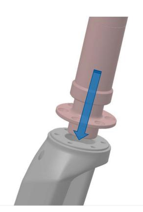
Align the suspension with the fork: the L mark (non-drive side) and R mark (drive side) must be aligned with the Left and Right bolt holes on the fork crown.
