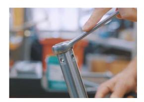
• The suspension will easily compress once the top cap has been loosened
