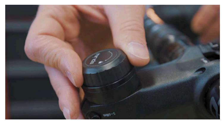
Test the function of the fork and check for potential play in the headset (with the fork locked out)
