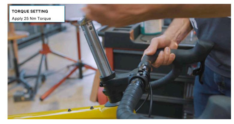
Tighten the top cap to 25 Nm using the 24mm wrench while keeping the suspension extended
