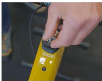
Remove the spring and Preload spacer attached using the magnet
